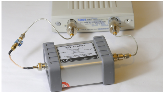
Figure 2: The 2-port setup with a 1 mΩ resistor for measurement.
